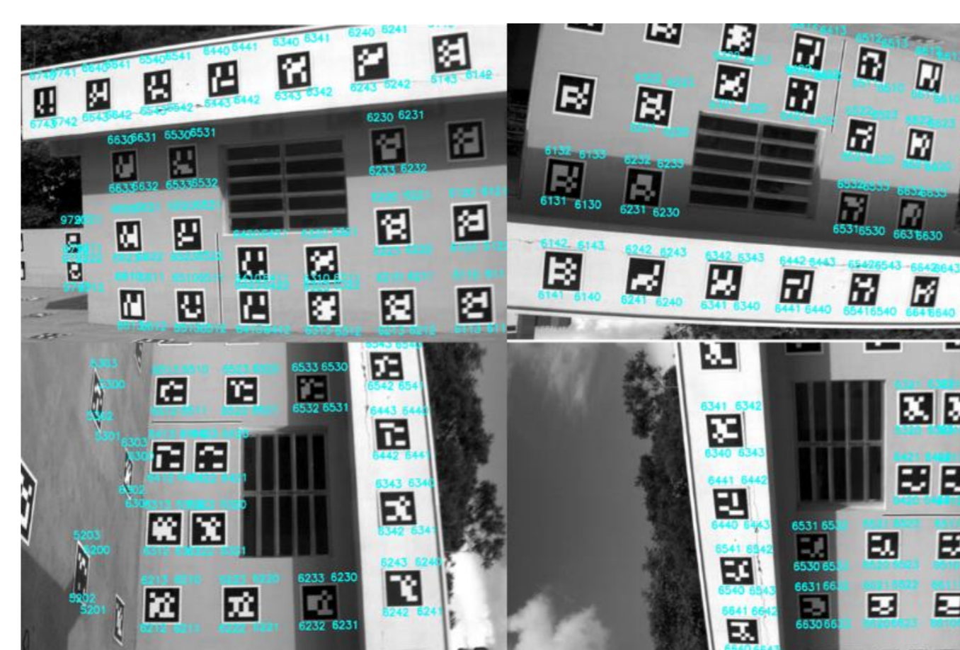
Sample of images acquired in the 3D terrestrial calibration field using the FPI camera.
